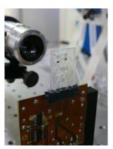
The FEMTO-ST Institute aims to develop a microrobot equipped with gripping capabilities moved and actuated remotely. The robot should be able to navigate in a blood sample to grasp a given cell, and bring it to a desired location for further biological analysis. This microrobot should be less than 1 millimeter long, biocompatible and vision based controlled.
