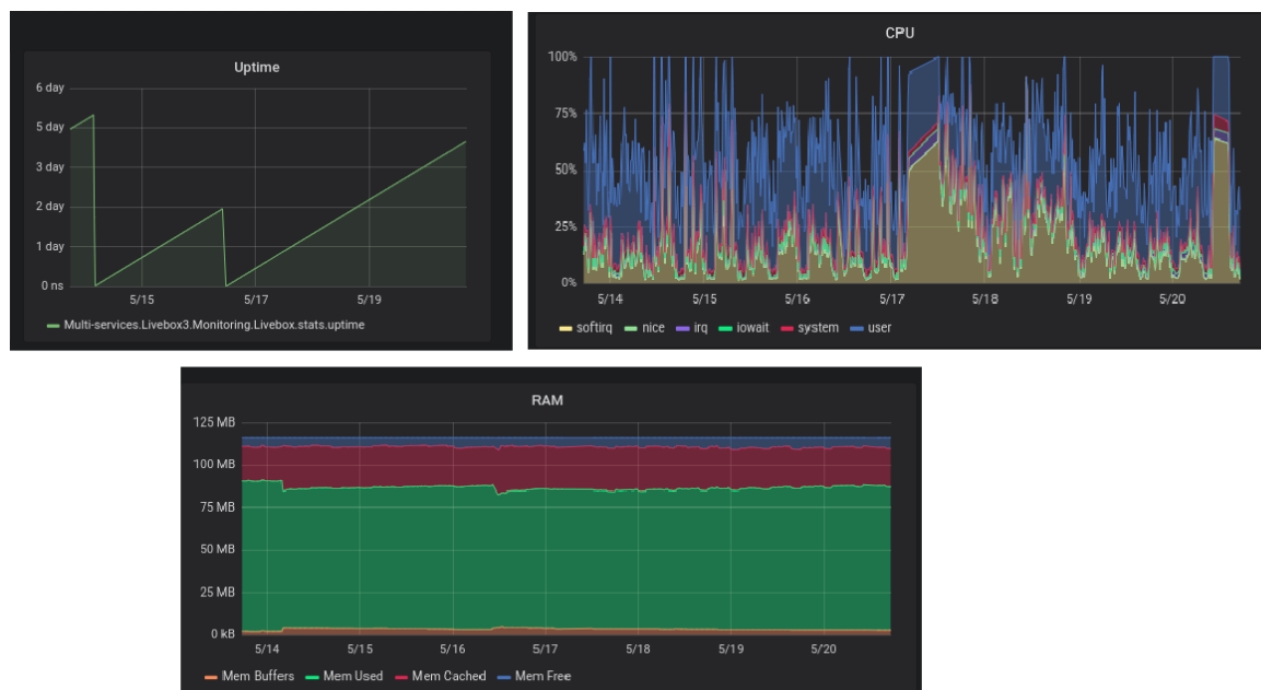
Figure 7 – Grafana screenshots showing uptime values, RAM and CPU status during a week
