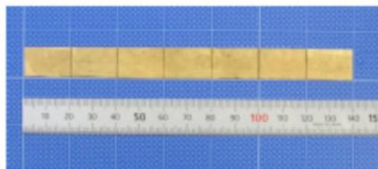
Figure 3. Beam-shaped IPMC actuator
