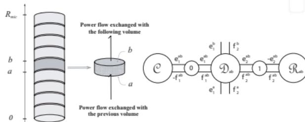
Figure 4: Principle of the spatial discretization
