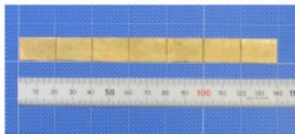
Figure 3. Beam-shaped IPMC actuator
